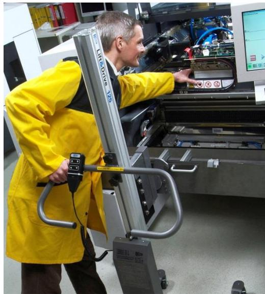
With a SIPLACE SX Capacity of Demand placement machine you can change a gantry in less than 30 minutes.
